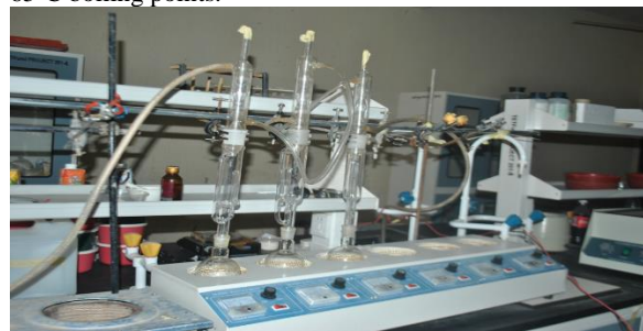
Plate 1: Soxhlet apparatus for fat determination (DHG-9023A, England)
